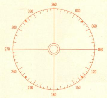
and stay on a given ADF bearing with Rose's help—no more mental gymnastics, such as relative bearing plus magnetic heading equals magnetic heading to the station, etc. . . . or how simple it becomes to figure the reciprocal of the published radial when you're inbound to MMM omni on Victor 10.
